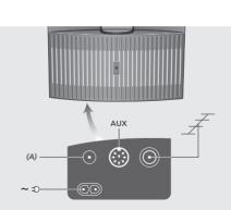
The socket panel is located underneath the BeoSound 1. The socket panel contains mains, aerial and AUX sockets.
